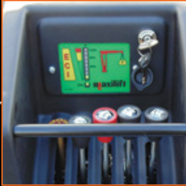
ECI: Electronic Capacity Indicator
