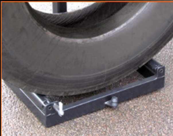
Lockable rollers for use when re-grooving
