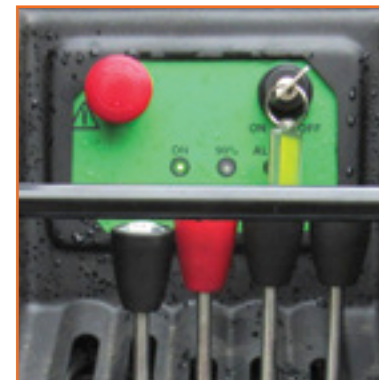
LME04: Load Limiting Device
