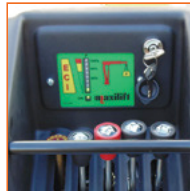
ECI: Electronic Capacity Indicator
