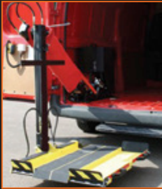
Automatic flaps ensure the load remains secure on the platform
