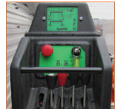
SCU: Stability Control Unit with LME04
